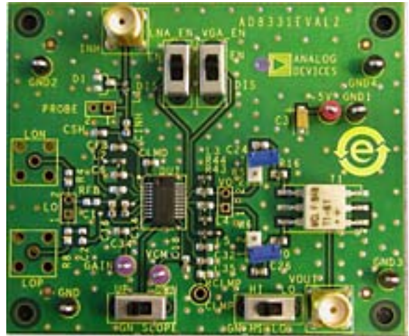
Figure 95. Photograph of AD8331-EVALZ
