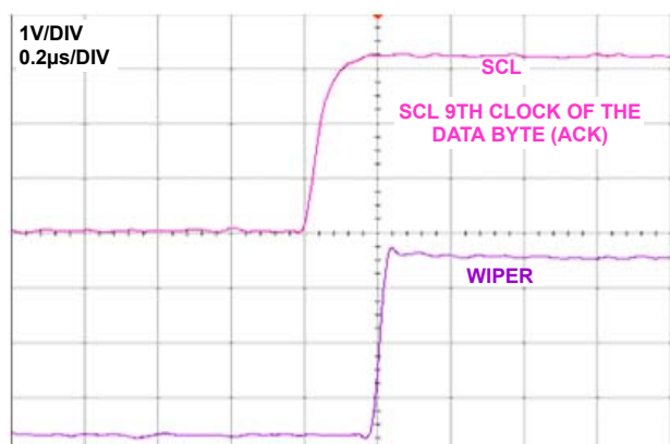
FIGURE 21. WIPER LARGE SIGNAL SETTLING TIME
