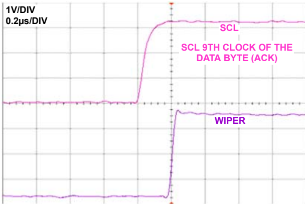
FIGURE 21. WIPER LARGE SIGNAL SETTLING TIME
