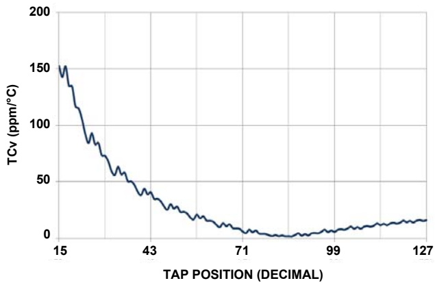
FIGURE 13. 10kΩ TCv vs TAP POSITION, V_{CC} = 3.3V
