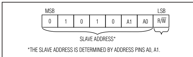
Figure 1. DS3502 Slave Address Byte
