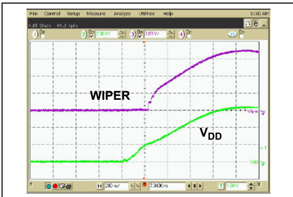
FIGURE 2-14: 2.1 k \Omega – Power-Up Wiper Response Time.
