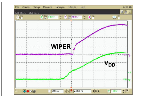
FIGURE 2-45: 50 k \Omega – Power-Up Wiper Response Time.
