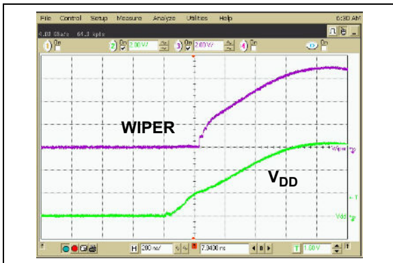
FIGURE 2-14: 2.1 k \Omega – Power-Up Wiper Response Time.
