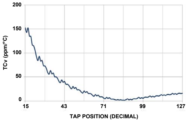
FIGURE 13. 10kΩ TCv vs TAP POSITION, V_{CC} = 3.3V
