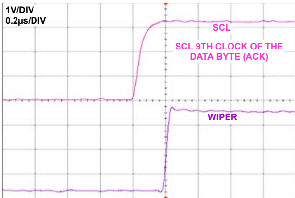
FIGURE 21. WIPER LARGE SIGNAL SETTLING TIME
