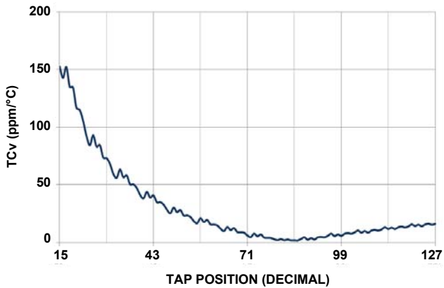
FIGURE 13. 10kΩ TCv vs TAP POSITION, V_{CC} = 3.3V
