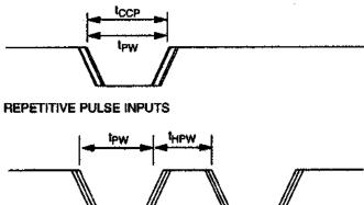
If during any pushbutton activity the STR input is activated, pushbutton operation will be suspended until the storage of EEPROM has been completed. Once complete, pushbutton inputs, if still active, will resume from the point of suspension. Command initiated storage operations will require a minimum of 4 ms to complete the storage operation. This 4 ms is measured from the rise of STR input (see Figure 5).
