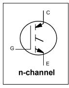
$V_{CES} = 600V$  $I_{C(Noml)} = 100A$  $V_{CE(on)} typ = 1.8V$ @  $I_{C(nom)}$ @ 25°C Motor Control IGBT Short Circuit Rated 150mm Wafer
