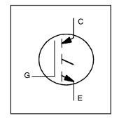
600 V  $I_{C(nom)} = 18A$   $V_{CE(on)} typ. = 1.65V @$   $I_{C(nom)} @ 25°C$ Motor Control IGBT
