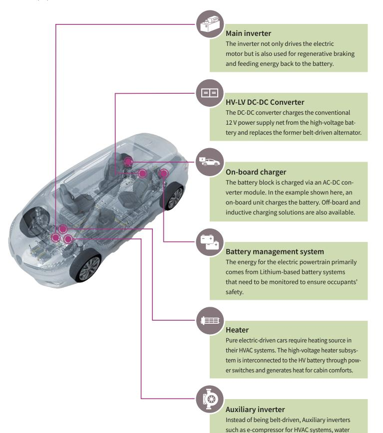
pumps, etc., are driven by electric power. Smart and energy-efficient auxiliary inverters are mainly realized through B6 bridges on its controller board.
