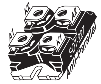
ISOTOP®[J] SOT-227 Antiparallel Configuration (Isolated Base)
