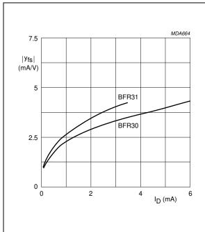
$V_{DS}$  = 10 V; f = 1 kHz;  $T_{amb}$  = 25 °C.
