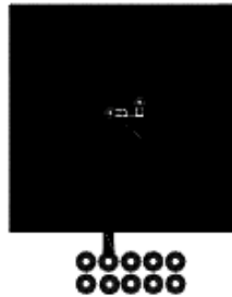
a. 52 ^\circ\text{C/W} when mounted on a 1 in 2 pad of 2 oz copper.
